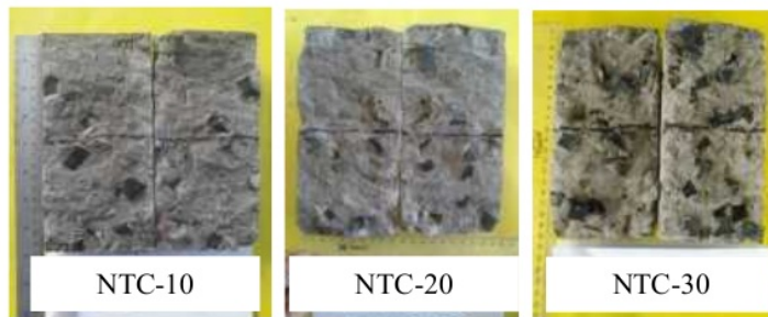
Figure 3. Tire chip detached from concrete paste.
